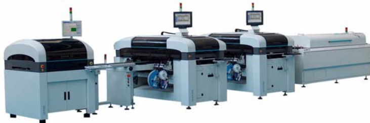
Megaflex assembly line with inline printer, HLX pick&places and full convection reflow oven (2006)
